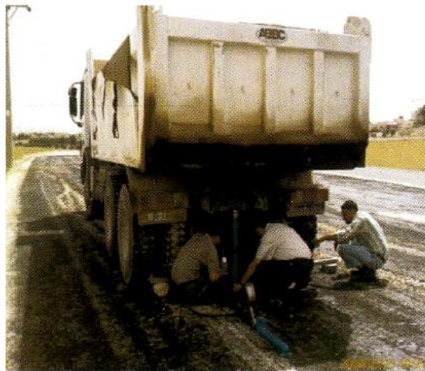
Fig. 8: Plate loading tests of the studied base material with different steel slag content
